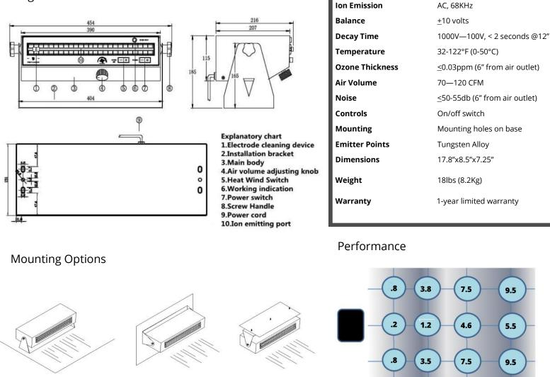
Testing was conducted in compliance with ANSI EOS/ESD S3.1-1991 of the ESD Association. Decay times in seconds. Distance in feet.
